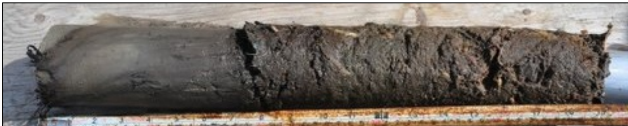
Typical core material from the northwest portion of the lake, with the organic material overlying the glaciomarine clay (note the organic material has compressed from approximately 0.6 m thick to 0.28 m during the coring process). The core top is to the right in the photo.
