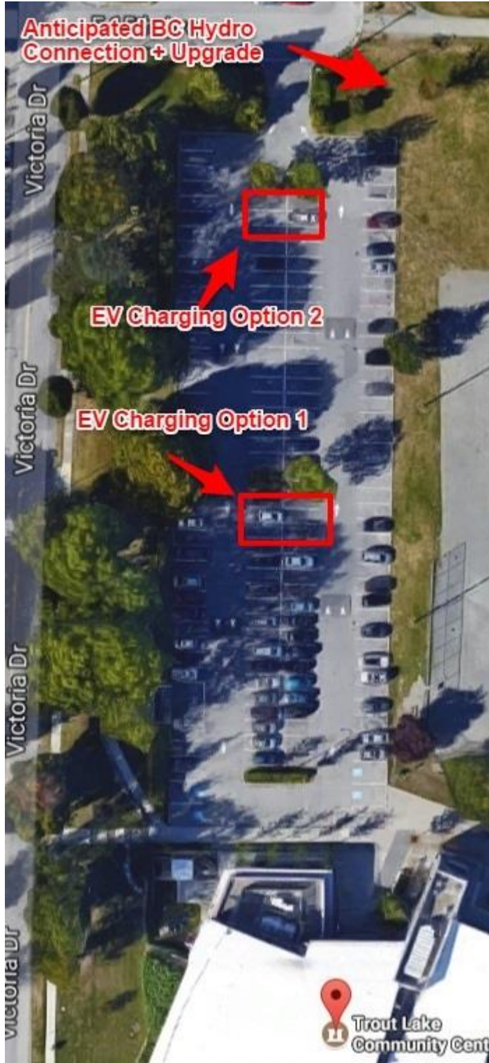
Figure 4 (left): Aerial photo showing the two proposed location options for EV charging infrastructure and approximate location of the anticipated tie-in with the BC Hydro distribution system.
