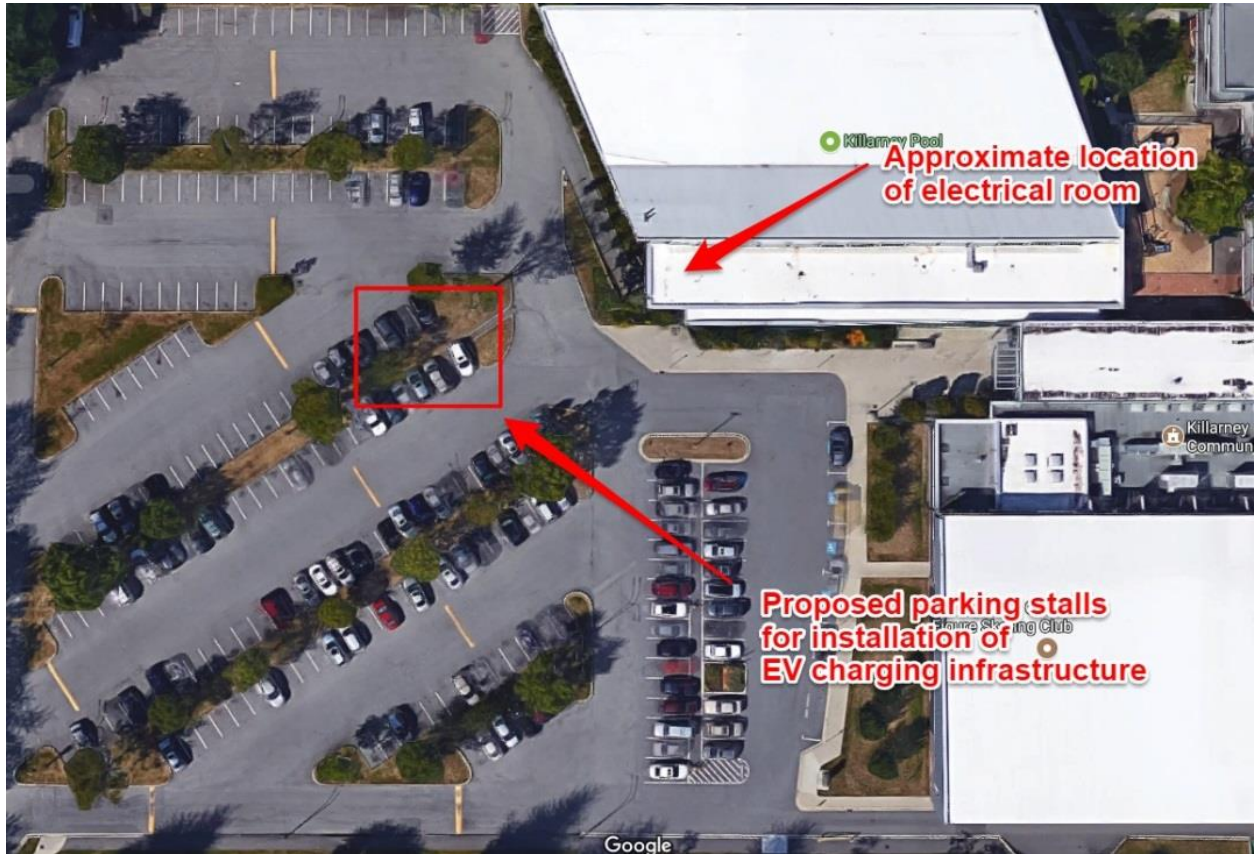
Figure 3 - Aerial photo showing proposed locations for EV charging infrastructure and approximate location of the building's electrical room.
