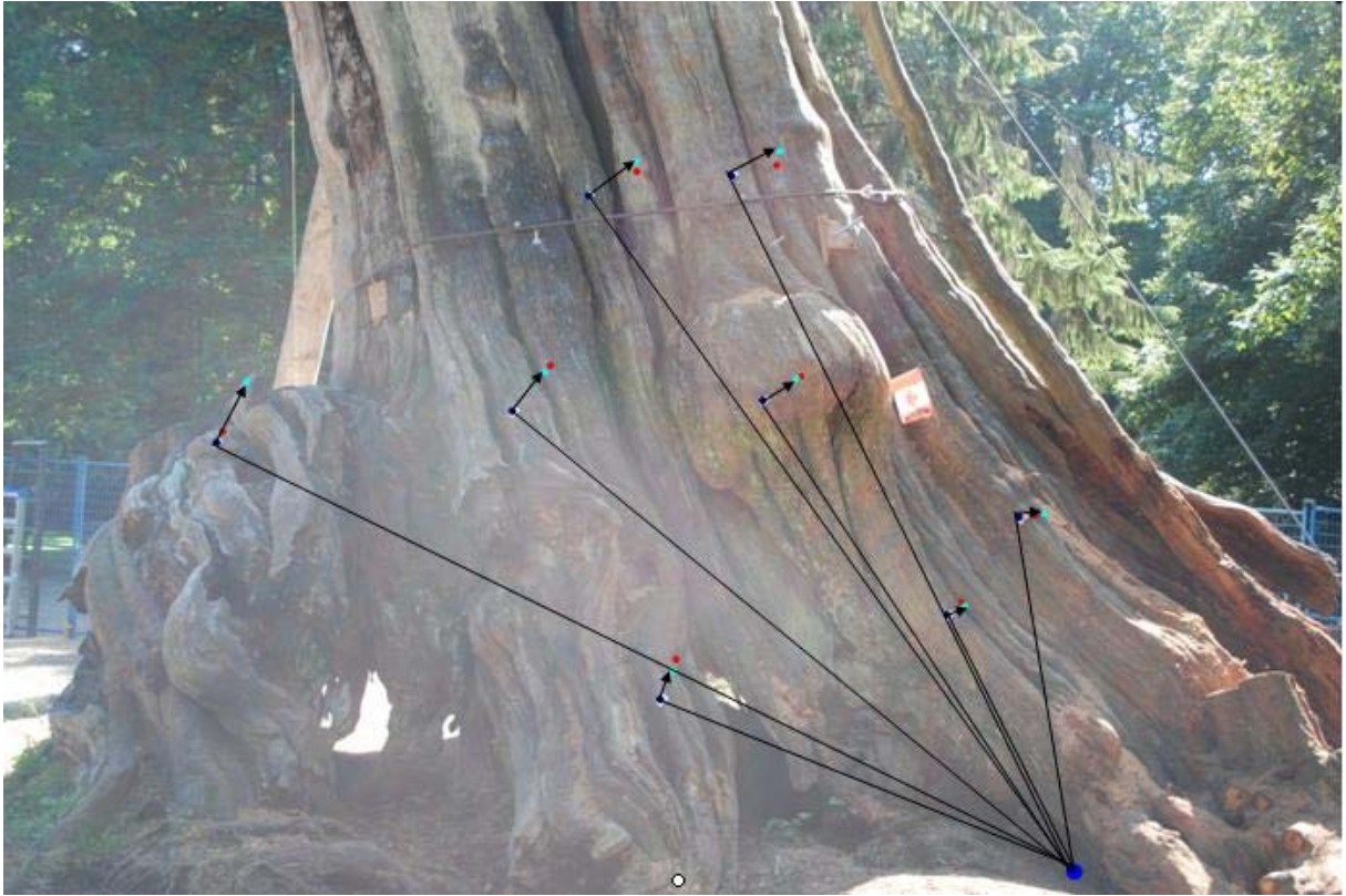
10X deflection representations. Red dots show observed displacement and the black arrows and cyan dots depict the best fit rotation.
