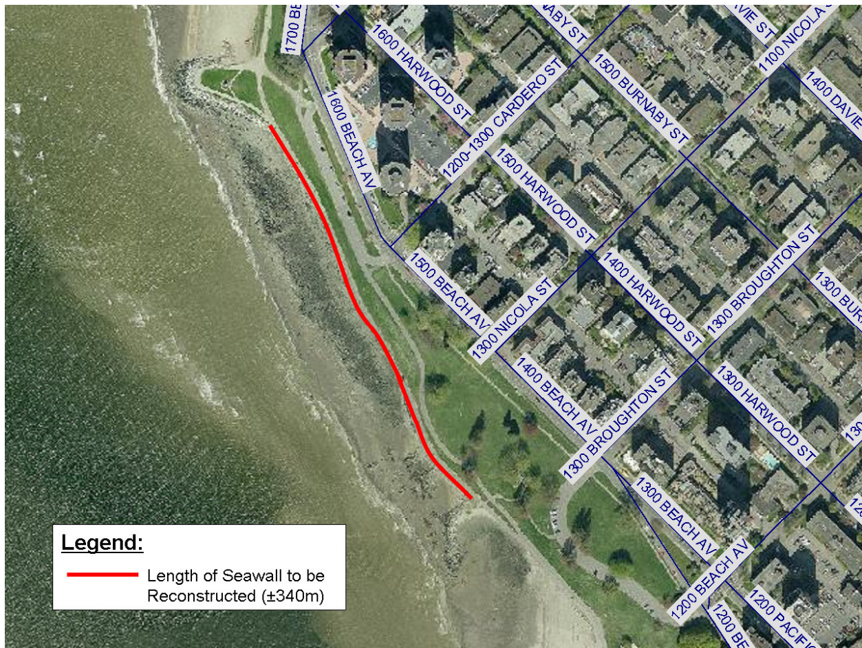
Figure 1: Length of seawall to be reconstructed at English Bay
