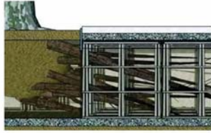
Illustration of Silva Cell tree system protecting tree roots and providing place for water infiltration
