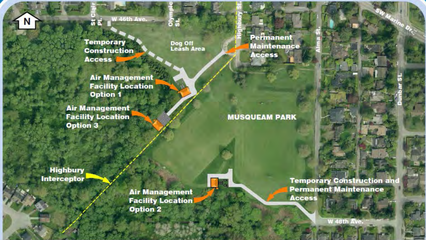
HIGHBURY INTERCEPTOR AIR MANAGEMENT FACILITY LOCATION OPTIONS 1, 2 & 3
