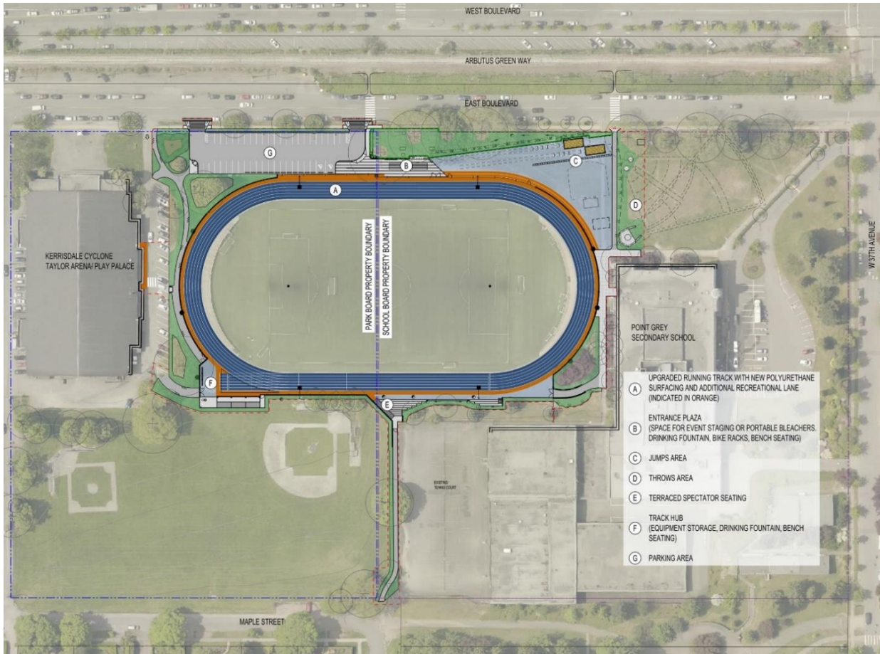
Figure 1: Concept Plan for Kerrisdale Park – Point Grey Secondary School Track and Field Upgrades. Surfacing areas indicated in dark blue, light blue and orange colouring.
