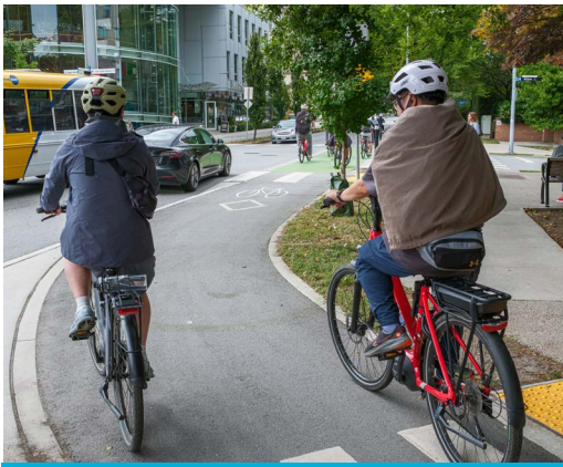
Chicane treatments are not common on bike paths but do exist where bike paths go from behind parking to curb side
