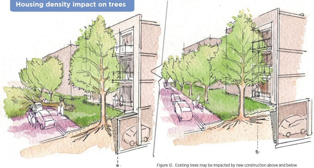
Figure 12. Existing trees may be impacted by new construction above and below ground when building or parkade setbacks are insufficient.
