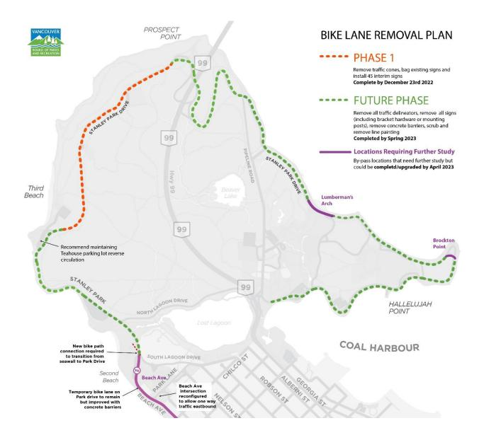
The total cost for the Phase 1 work is \$25,000 which includes drawings and stamp by the Engineer of Record (EoR), fabrication and installation of new interim signage, removal of the cones, and final EoR inspections and sign off.
