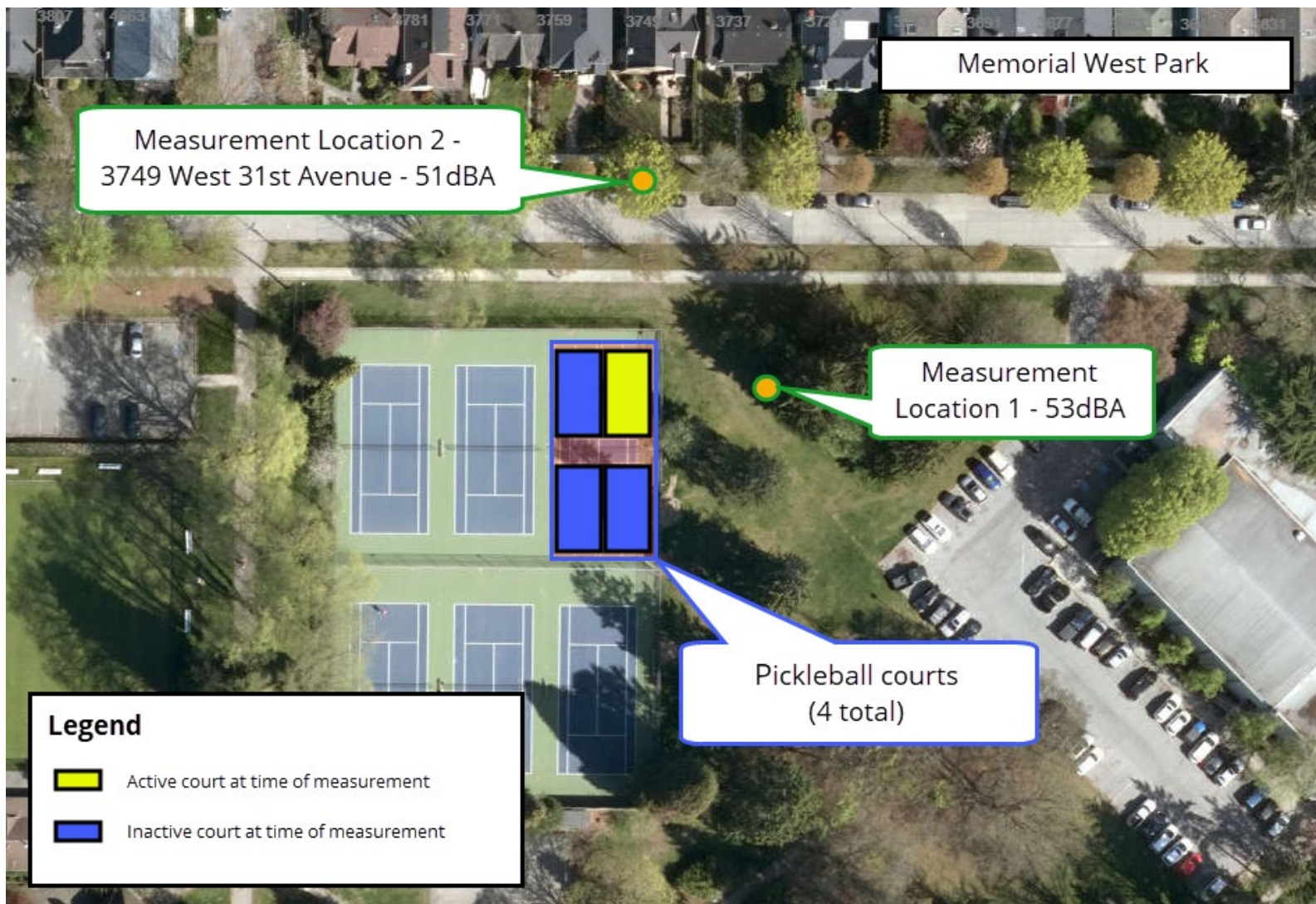
Figure 2: Memorial West Park Pickle Ball Courts and Measurement Locations
